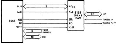
another using standard MCS-80/85 I/O devices; and a third using the combination memory/I/O expander devices the 8155, 8355, and 8755. It is also possible to expand using standard TTL devices as shown in Chapter 5.
